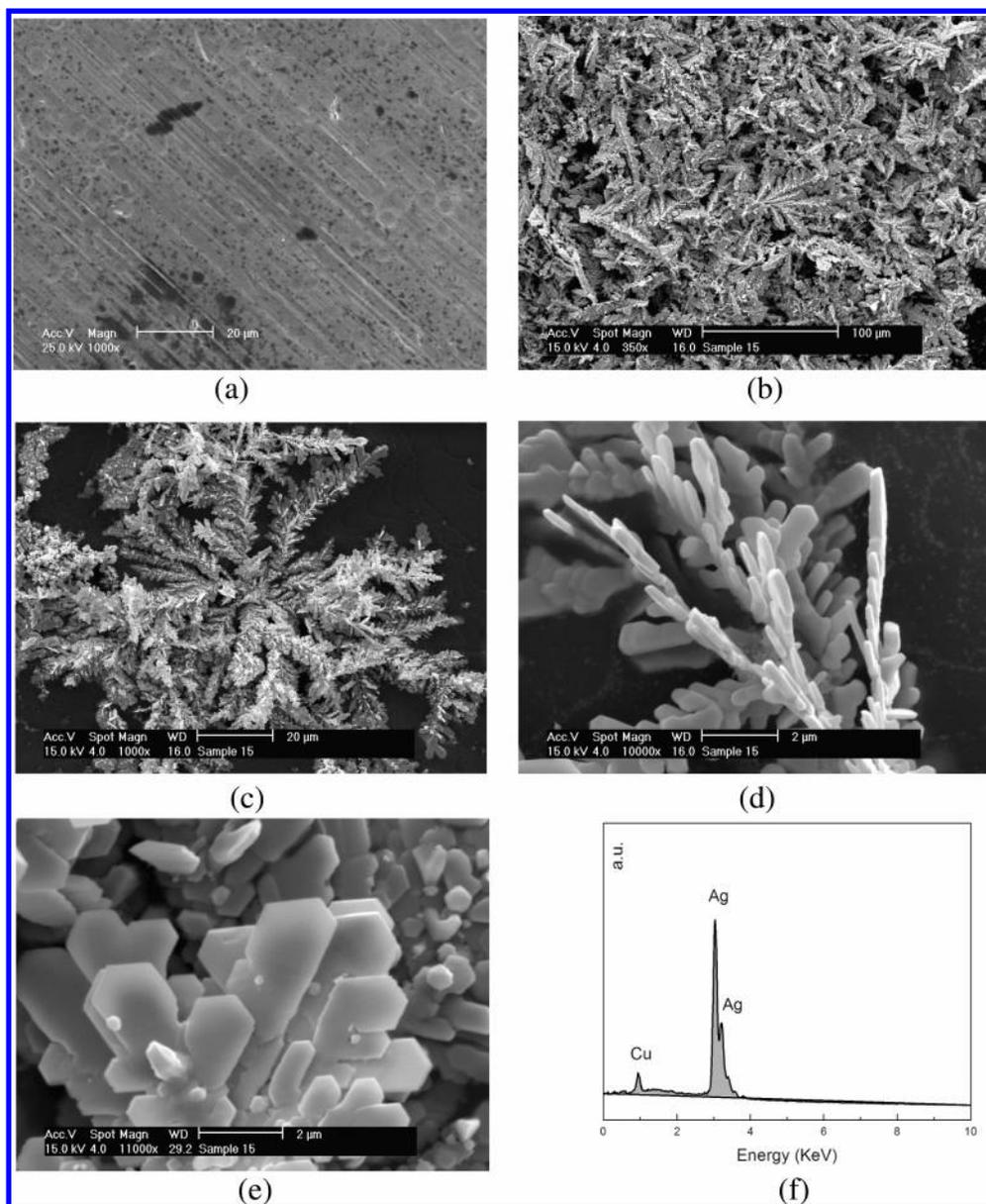
**Figure 2.** SEM images of (a) surface of the Cu foil, (b,c) leaflike silver microstructures formed on the Cu surface, (d,e) as for (c) taken from different areas under a higher magnification, and (f) EDX spectrum of the silver nanoclusters.
