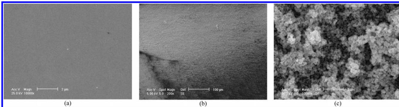
**Figure 1.** SEM images of (a) smooth glass plate, (b) silver nanostructures deposited on the glass surface, and (c) as for (b) under a higher magnification.
