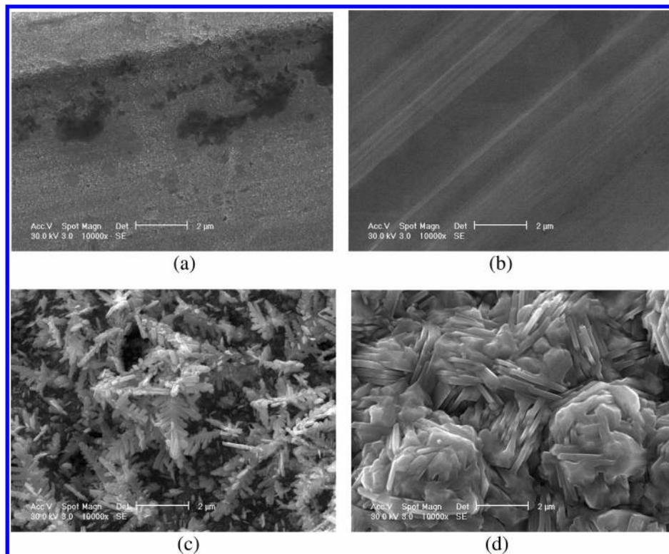
**Figure 6.** SEM images of Cu foils treated with an aqueous solution of HCl (0.5 M) for (a) 5 min and (b) 60 min, and silver nanostructures from the silver mirror reaction on the corresponding Cu foils (c) for (a) and (d) for (b).
