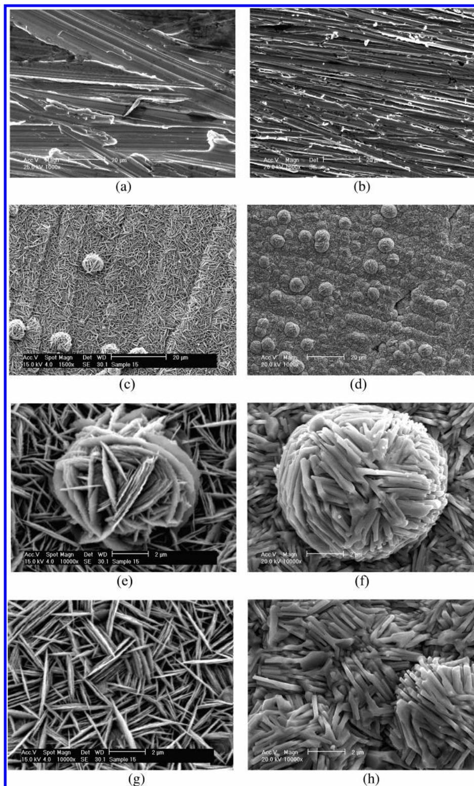
**Figure 5.** SEM images of Cu foils rubbed with the (a) 180-C and (b) 600-B sandpapers, and silver nanostructures from the silver mirror reaction on the corresponding Cu foils (c,e,g and d,f,h for the 180-C and 600-B sandpaper-rubbed Cu substrates, respectively) under different magnifications.
