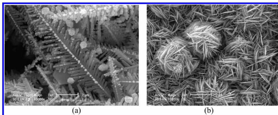
**Figure 7.** SEM images of silver nanostructures formed by reacting (a) a commercially available Cu foil with an aqueous solution of  $\text{AgNO}_3$  ( $6.375 \times 10^{-3}$  M), and (b) a sandpaper (180-c)-rubbed Cu foil with an aqueous solution of  $\text{Ag}(\text{NH}_3)_2^+$  ( $6.375 \times 10^{-3}$  M).
